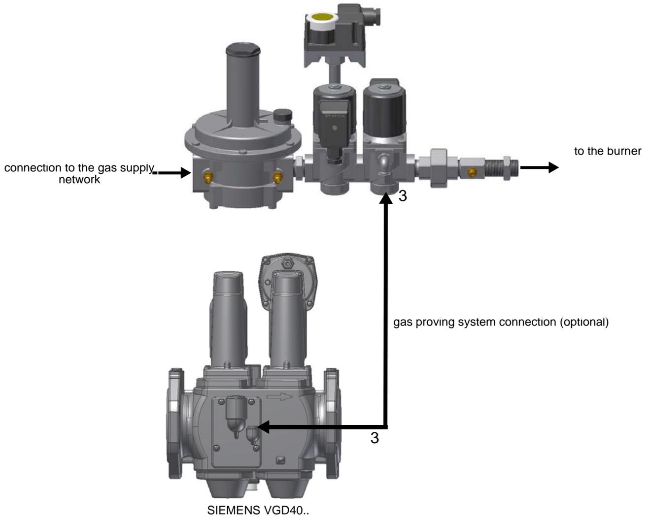
Fig. 5 - pipe port (3) for connecting the pilot gas train to the valves group of the main gas train
