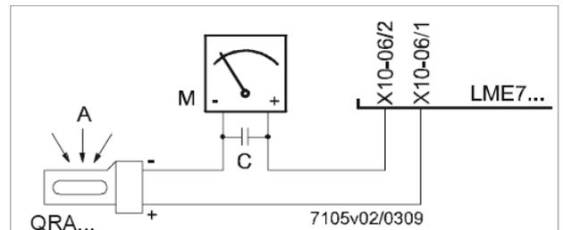
Fig. 18: Detection by photocell QRA..
