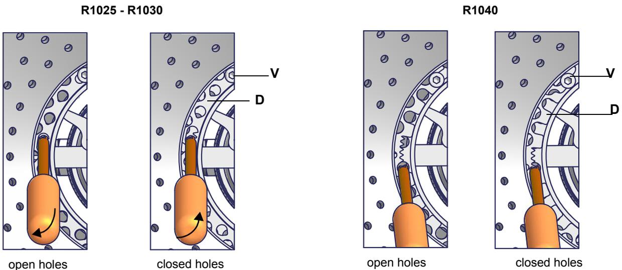
The adjusting plate correct position must be regulated in the plant during the commissioning. The factory setting depends on the type of fuel for which the burner is designed:
