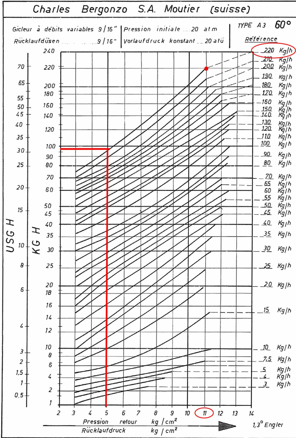
**Example (Bergonzo):** if a 220kg/h flow rate BERGONZO nozzle is provided, set the return pressure at 11bar, supply at 20bar on the delivery to get a 220kg/h flow rate. If the return pressure needed is 5bar, instead, act on the **V** adjusting screw on the pressure governor. The flow rate will then be about 95kg/h (see the example showed on the Bergonzo diagram).
