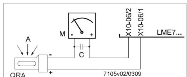
Fig. 24: Detection by photocell QRA..
