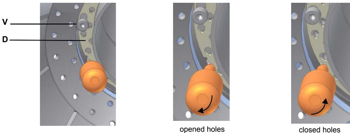
The adjusting plate correct position must be regulated in the plant during the commissioning.
