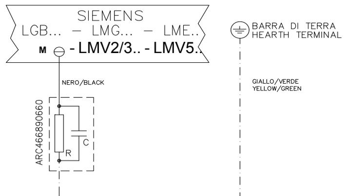
For LMV5 control box, please refer to the labeling recommendations available on the Siemens CD attached to the burner
