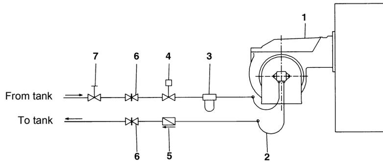
Fig. 16 - Double-pipe system
