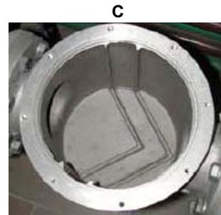
**Inspection and replacement of the MULTIBLOC DUNGS MBC..SE filter (Threaded valves group)**
