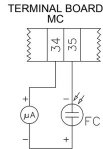
Fig. 37: Detection by photocell QRA..
