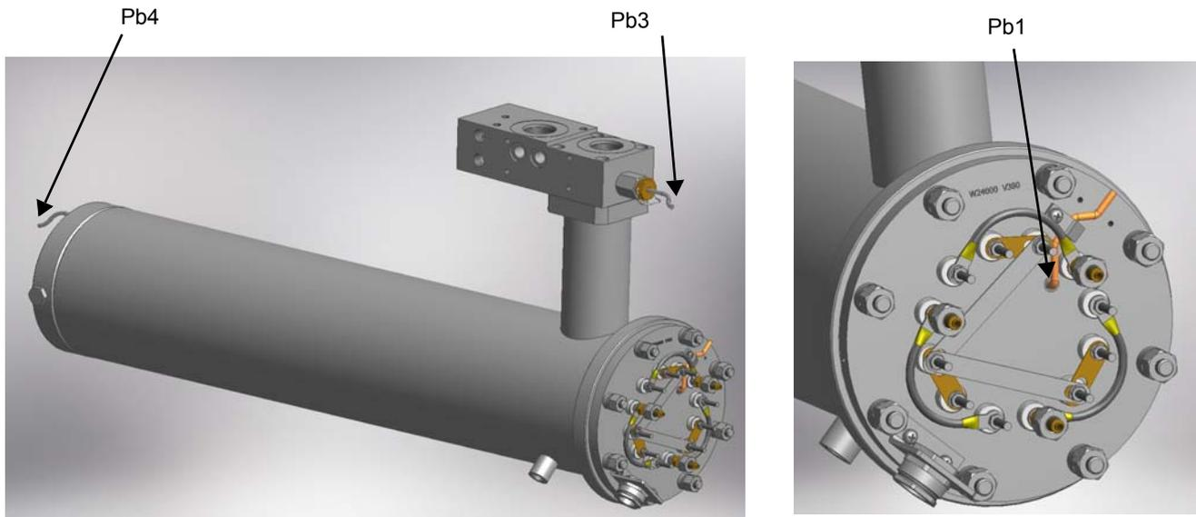
Fig. 29 - Probe connections (Danfoss MCX)
