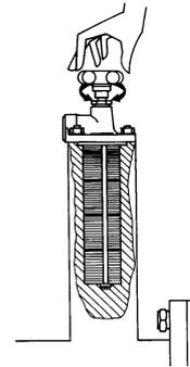
**Replacing the spring in the gas valve group**
