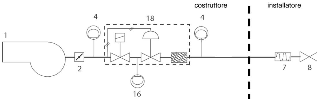
Gas train with valves group MBC SE1900/3100/5000 (2 valves + gas filter)+ press. governor + PGCP gas proving system pressure switch
