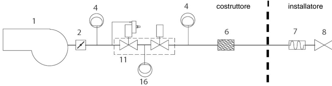
Gas train with valves group MBC SE1200 (2 valves + gas filter + press. governor) + PGCP gas proving system pressure switch
