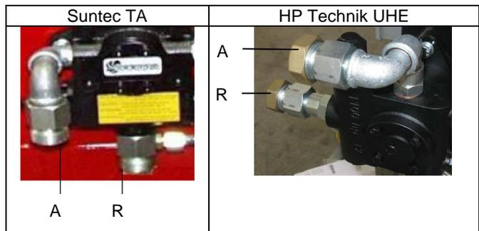
**Connecting the burner to the oil pumping unit**
