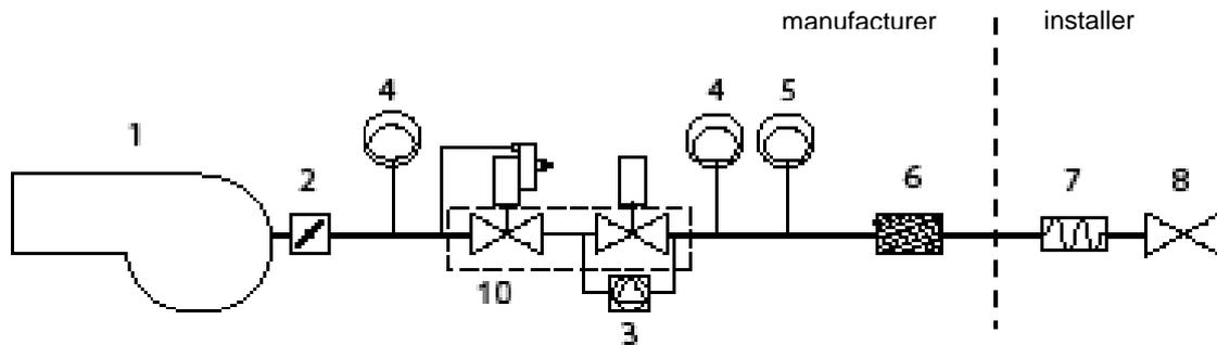
Gas train with valves group MBC 1200SE (2 valves + gas filter + pressure governor) + VPS504 gas proving system
