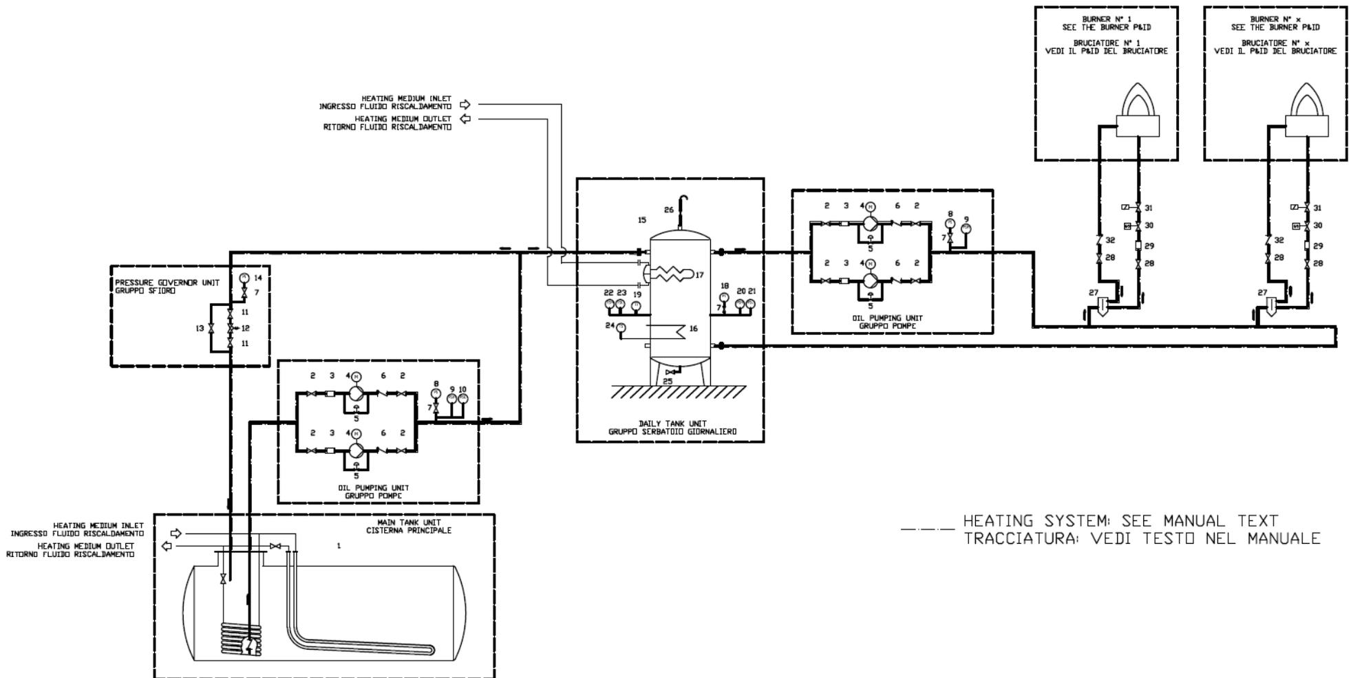
Fig. 11 - Two or more burners configuration
