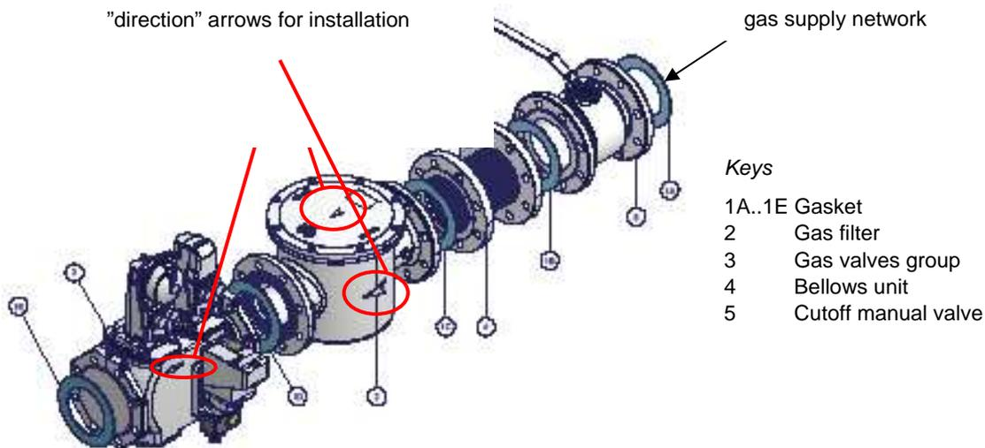
Fig. 4 - Example for gas train
