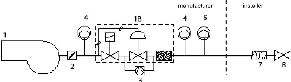
Gas train with valves group MBC 1900/3100/5000SE (2 valves + gas filter) + pressure governor + VPS504 gas proving system
