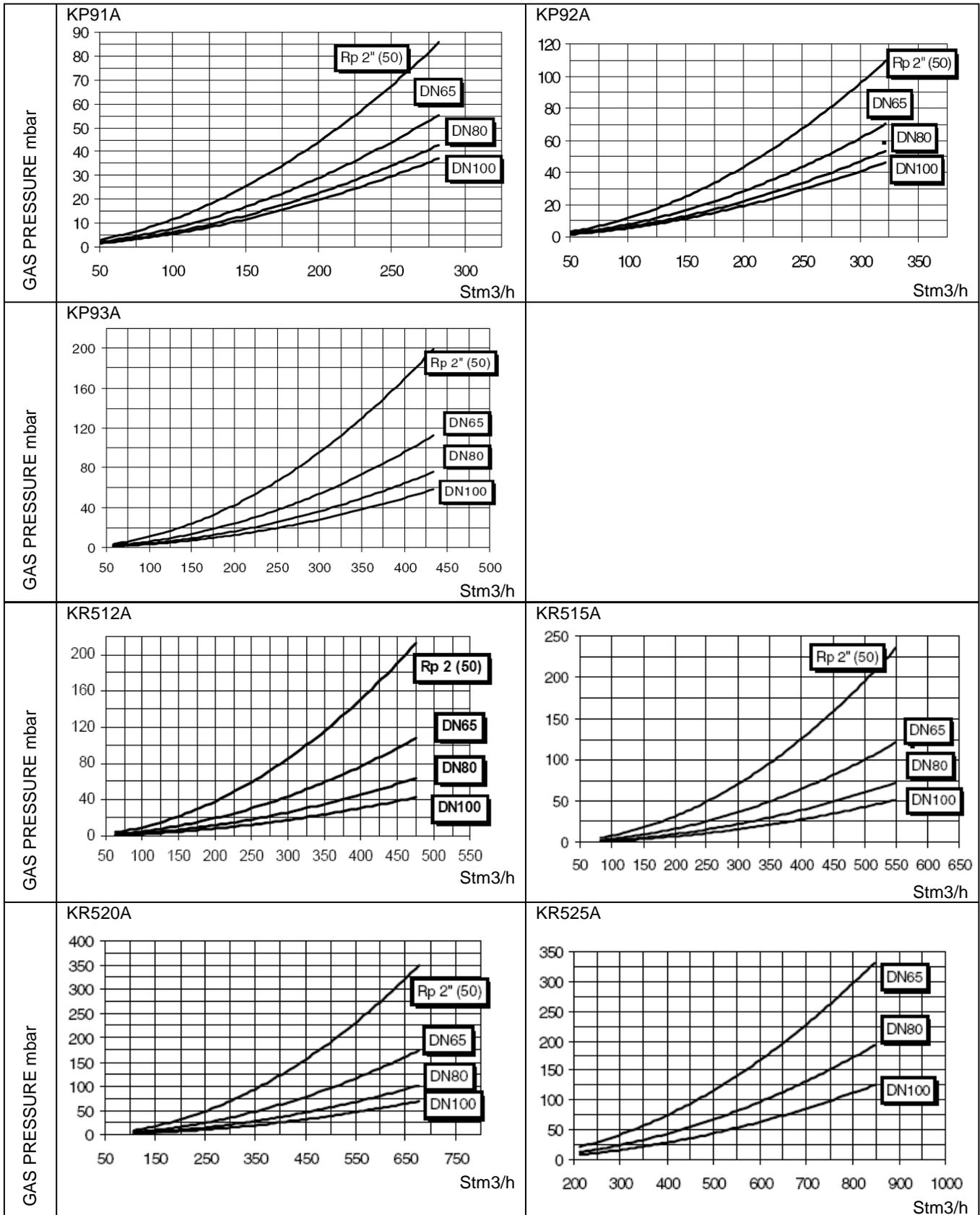
**Caution:** the gas rate value is quoted on the x-axis, the related network pressure is quoted on the y-axis (pressure value in the combustion chamber is not included). To know the minimum pressure at the gas train inlet, necessary to get the requested gas rate, add the pressure value in the combustion chamber to the value read on the y-axis.
