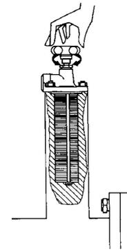
**Removing the combustion head**
